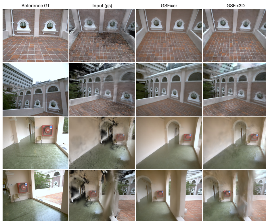
Figure 12. Novel view repair on a challenging outdoor scene from the FAST-LIVO dataset [41]. The initial reconstruction is generated by a LiDAR-Inertial-Camera Gaussian Splatting SLAM system [11], which may contain pose errors and produce inaccurate maps. Our method manages to repair those broken geometries to some extent.
